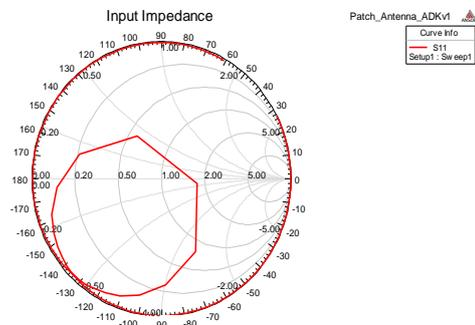
Fig.3. Smith chart of single band microstrip antenna at 3 GHz
