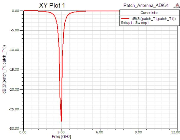
Fig.2. Simulated returns loss of single band antenna at 3 GHz
