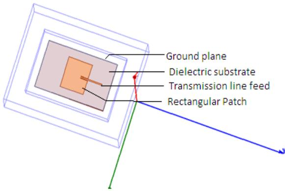
Fig.1. Geometry of desired single band microstrip patch antenna
