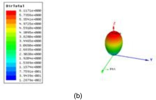
Fig.4. Directivity of single band antenna at 3 GHz (a) 2D Pattern (b) 3D Pattern
