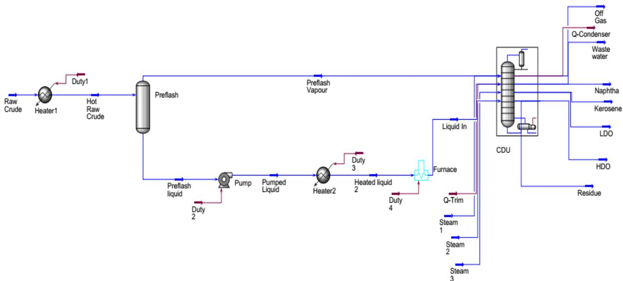
Figure 3: Simulation Diagram of the Atmospheric Distillation Unit
