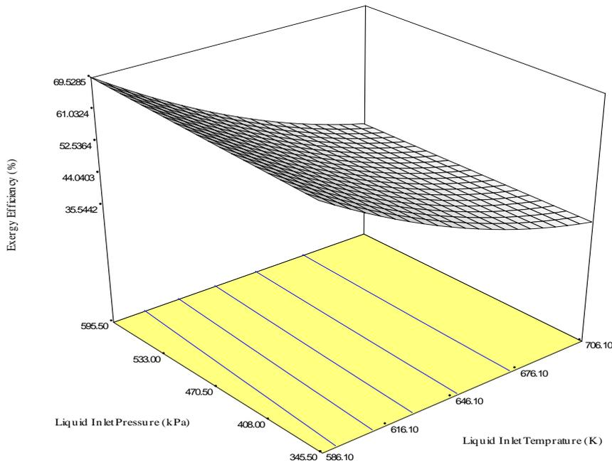
Figure 6: 3-D Response Surface Map for AC (liquid inlet temperature and condenser pressure) Combination [14]
