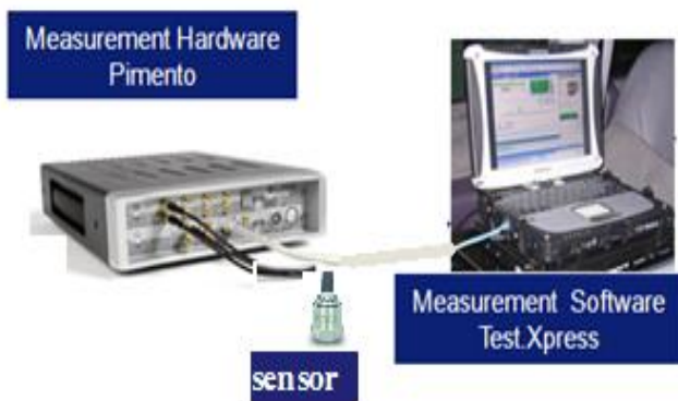
Figure 4: Typical setup of transducer-data acquisition pair
