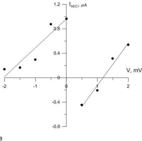
Fig. 1. Dependences of  $I_{AEC} f(V_{bias})$  under the influence of SAW with a frequency  $f = 54,2$  MHz is shown at various  $I_{SAW}$ : a)  $I_{SAW} = 0 \mu A$ ; b)  $I_{SAW} = 25 \mu A$ ; c)  $I_{SAW} = 50 \mu A$ ; d)  $I_{SAW} = 75 \mu A$ ; e)  $I_{SAW} = 100 \mu A$ . Power SAW source  $W = 1.07 Wt$ .
