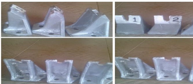
Plate 1:Aluminium casting of engine sittings for Peugeot 504 cars from Okenya (1), and Okenya with Shea Butter (3)
