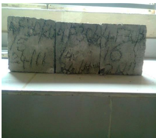
Plate 2. Ductile (non explosive) failure of sisal fibre reinforced concrete cube specimen.
