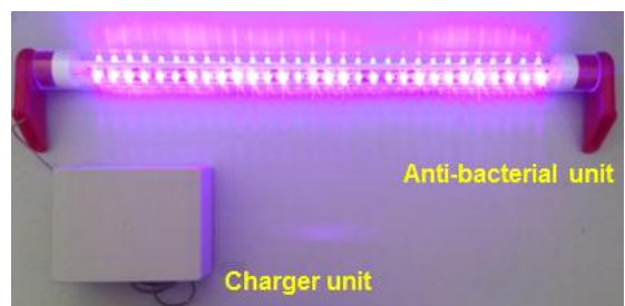
Figure 2 - Anti-bacterial shopping cart handle prototype.
