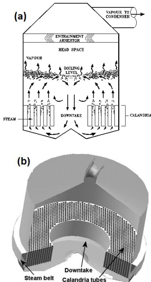
Fig. 1 Batch vacuum pan (a) Circulation patterns and (b) Sectioned view [2]
