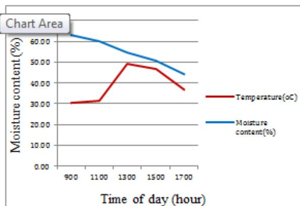
Fig. 5: Effect of temperature and air circulation on drying rate (half opened inlet)
