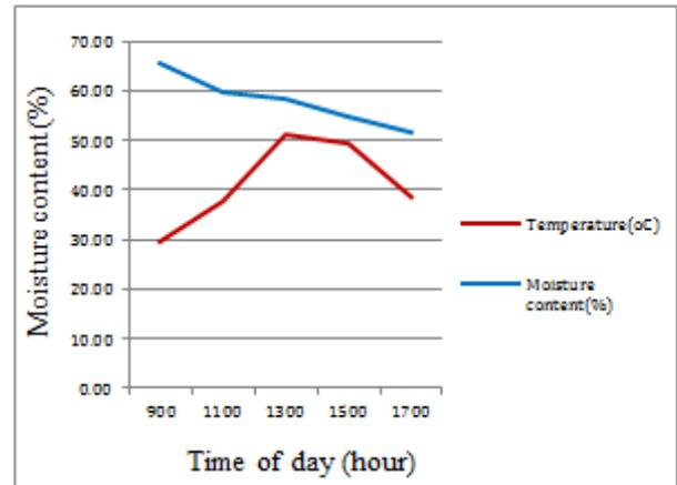
Fig. 6: Effect of temperature and air circulation on drying rate (totally closed inlet)
