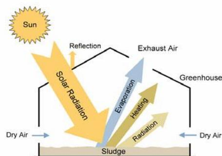
Fig. 1: Basic principle of solar dryer. Reference [3]
