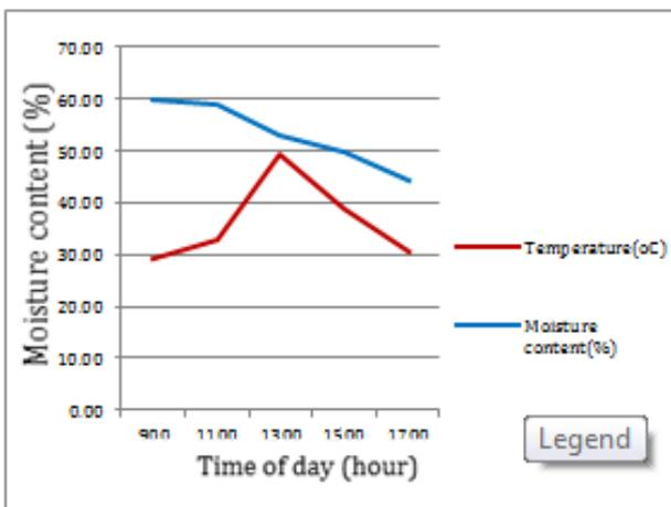
Fig. 4: Effect of temperature and air circulation on drying rate (fully opened inlet)
