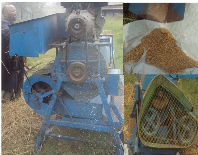
Fig. 2. Fadis research center multi crop thresher
