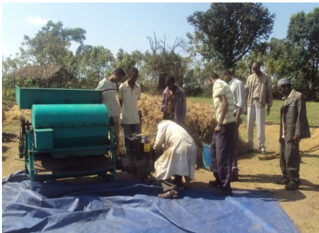
Fig. 1. Assela model 2 Axial Flow multi crop thresher
