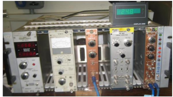
Fig4 Sets of photon counting electronics used in the experiments.
