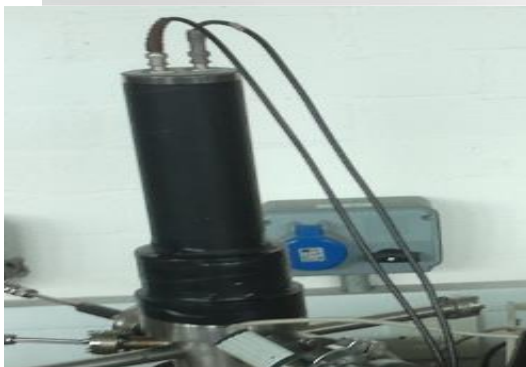
Fig 3 The 9813QA, Thorn EMI photomultiplier tube before and during use.
