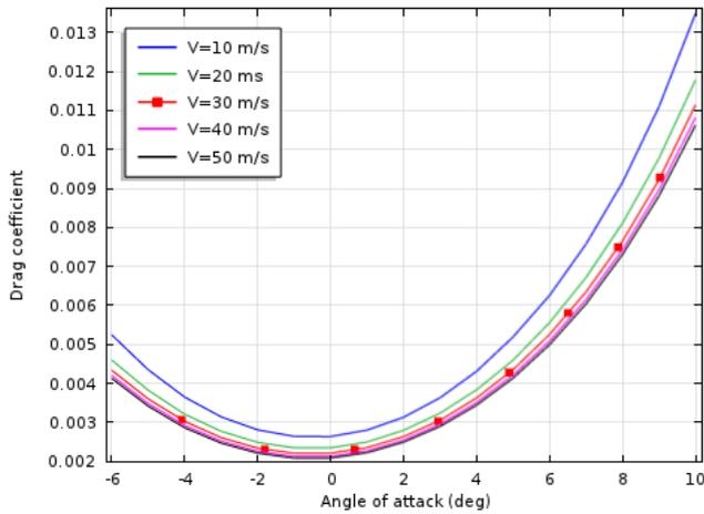
Figure 4. Drag coefficient versus angle of attack
