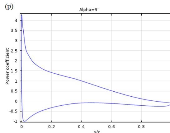
Figure 6a-r. Pressure coefficient of NACA NACA 632-215 airfoils with different angle of attack.
