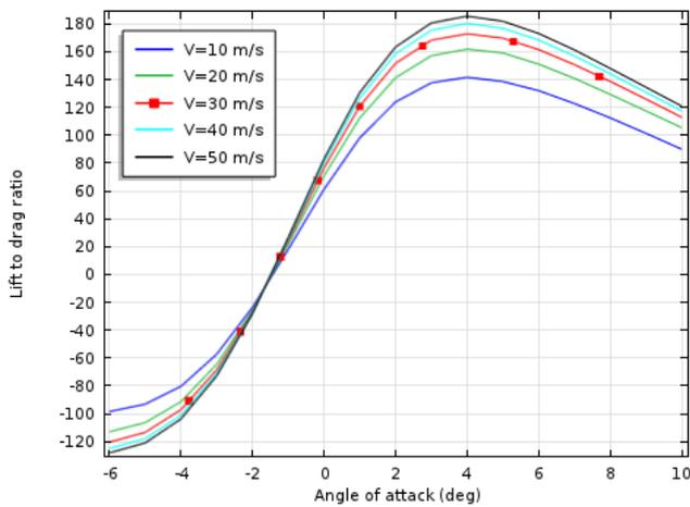
Figure 5. lift to drag ratio versus angle of attack
