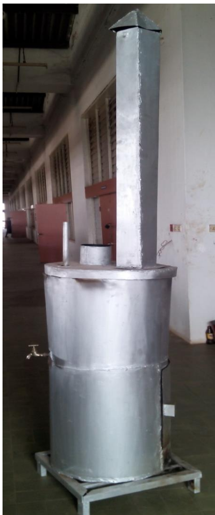
Fig. 2: Picture of the Domestic Water Heating Solid Waste Incinerator
