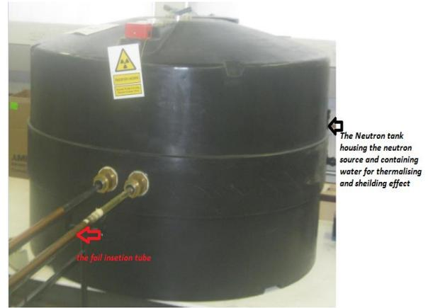
Fig 4 snapshot of the neutron tank in Manchester laboratory used for the modelling.
