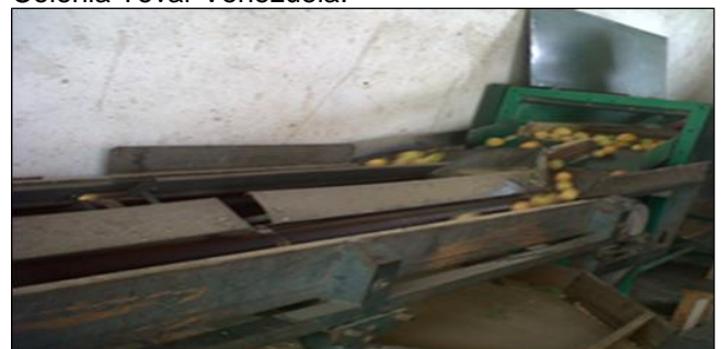
Figure 2. A machine that removes the outer hair peach.
