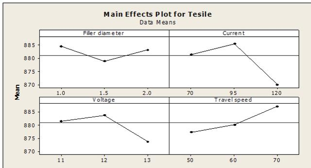
Fig. 4. Main effect plots for welding parameters via tensile strength
