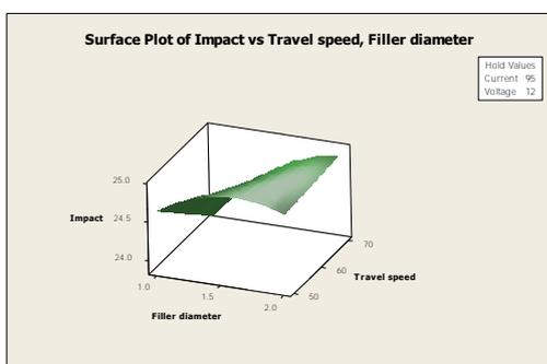
Fig. 18. Contour plot of impact force via travel speed, filler diameter
