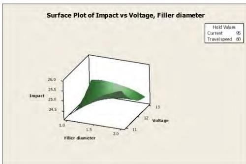
Fig. 17. Contour plot of impact force via welding voltage, filler diameter
