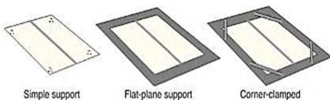
Fig. 2. supporting for butt welding
