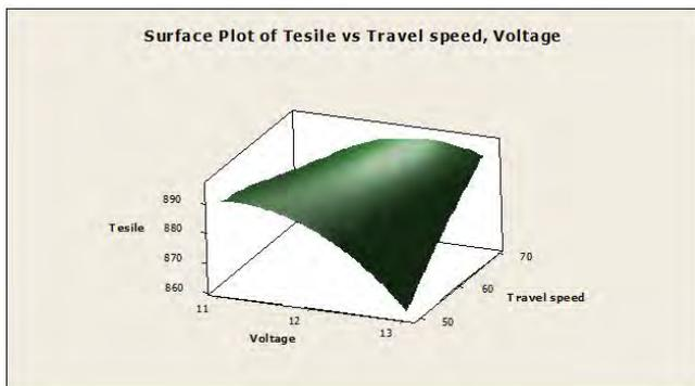
Fig. 5. Contour plot of tensile strength via welding voltage, travel speed
