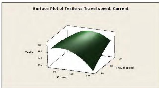
Fig. 6. Contour plot of tensile strength via welding current, travel speed
