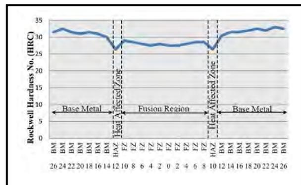
Fig. 20. Relationship between Hardness No. and the (BM, HAZ, FZ) regions in Ti-6Al-4V weldment
