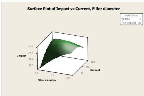
Fig. 16. Contour plot of impact force via welding current, filler diameter
