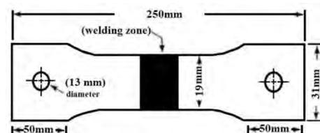
Fig. 3. Tensile sample
