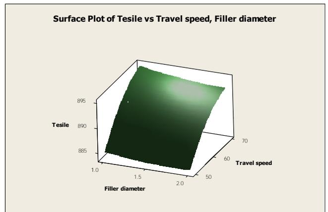
Fig. 8. Contour plot of tensile strength via filler diameter, travel speed
