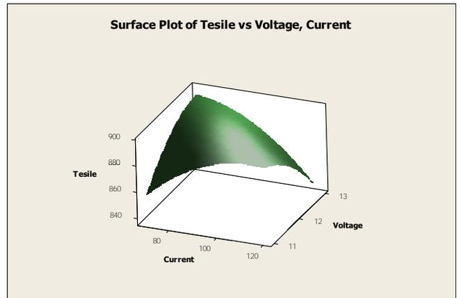
Fig. 7. Contour plot of tensile strength via welding current, welding voltage.
