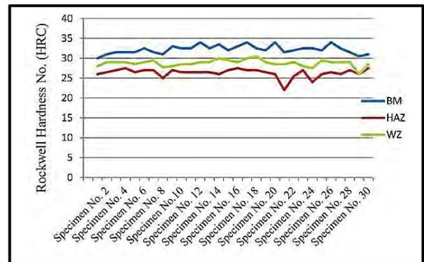
Fig. 19. Rockwell Hardness No. (HRC) for the BM, WZ, and HAZ in Ti-6Al-4V weldment
