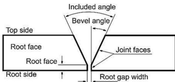
Fig. 1. joint with edges preparation
