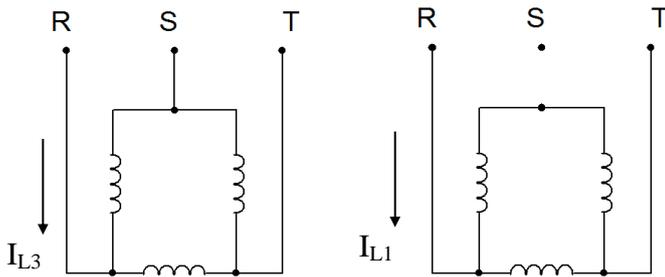
Fig. 5. Delta Connected Windings at Normal Supply and at Single Phasing
