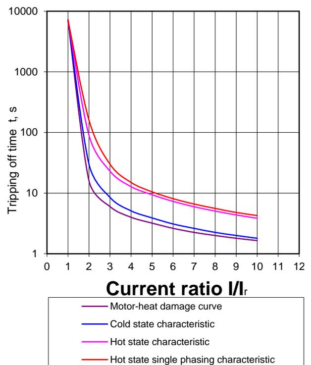
Fig. 2. Bimetal Time-Current Characteristics
