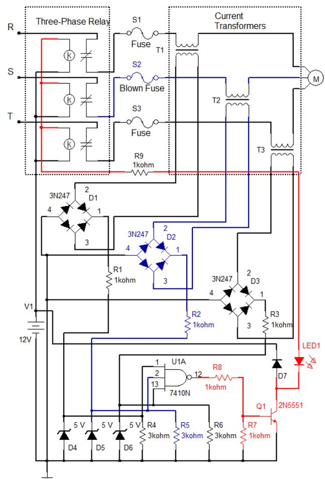
Fig. 7. Single Phasing Protection
