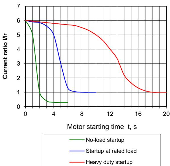
Fig. 3. Current Characteristics at Different Loads
