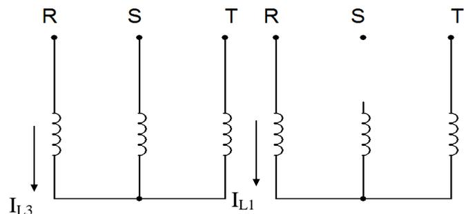
Fig. 4. Star Connected Windings at Normal Supply and at Single Phasing
