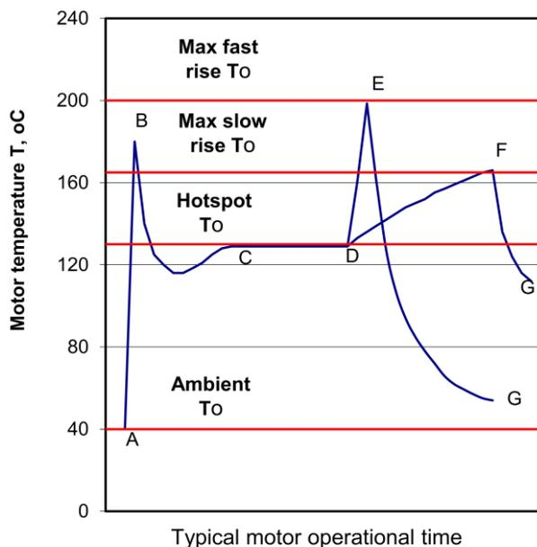
Fig. 1. Typical Temperature Characteristics
