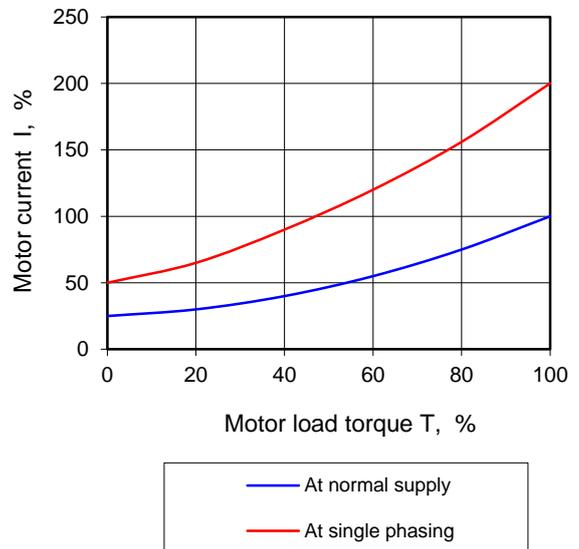
Fig.6. Current-Load Characteristics
