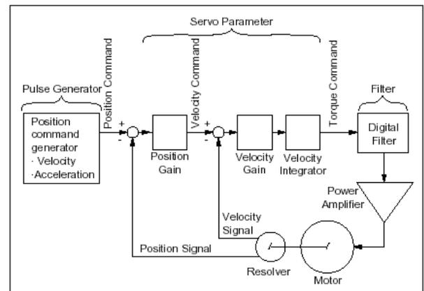
Fig. 4. Control position system of the brushless
