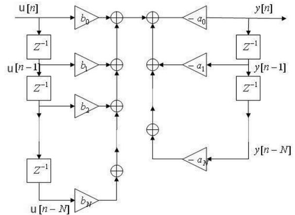
Fig. 1. Block diagram of an LPC gaussian model.
