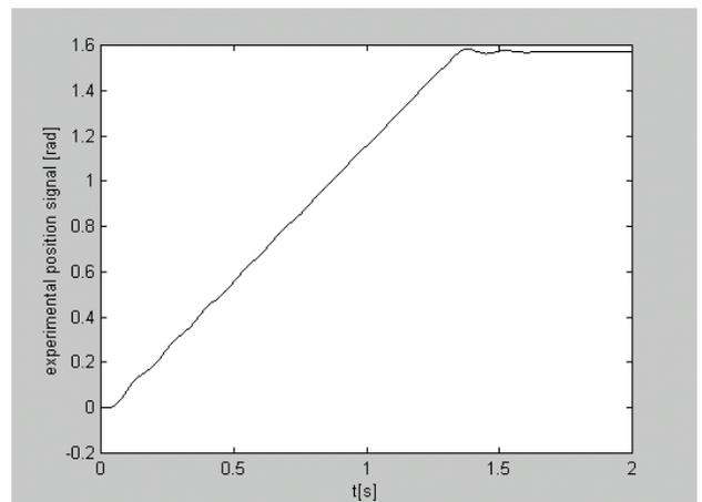
Fig. 15 Experimental angular position of the brushless motor
