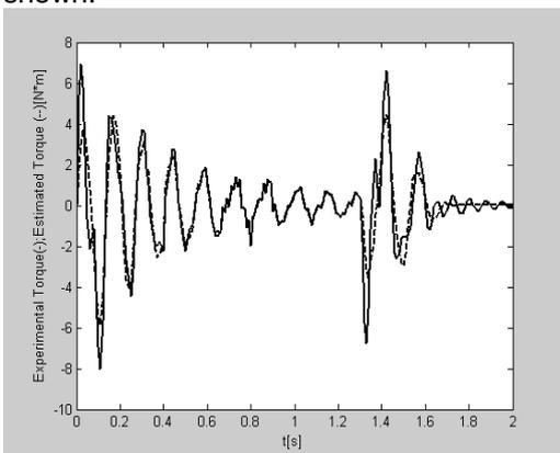
Fig. 13 Experimental torque command (-), estimated torque command (-) [Nm]
