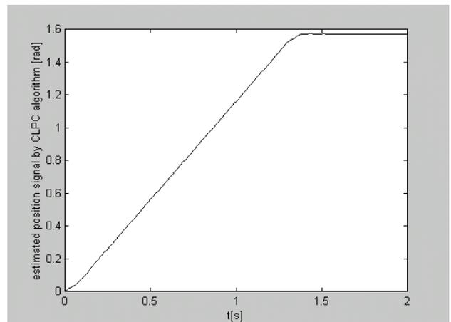
Fig. 16 Estimated angular position signal of the brushless motor
