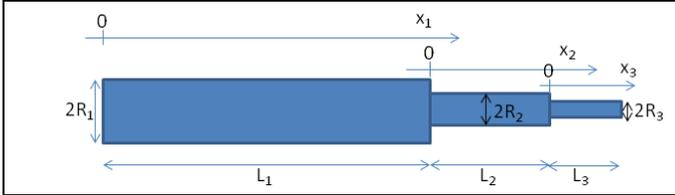
Fig.2. Schematic of the two-step ended rod.
