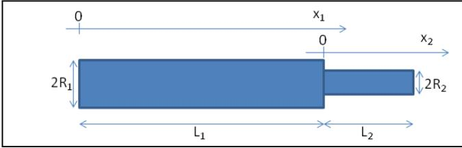
Fig.2. Schematic of the one-step ended rod.
