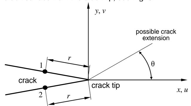
Fig. 5. Displacement correlation method
