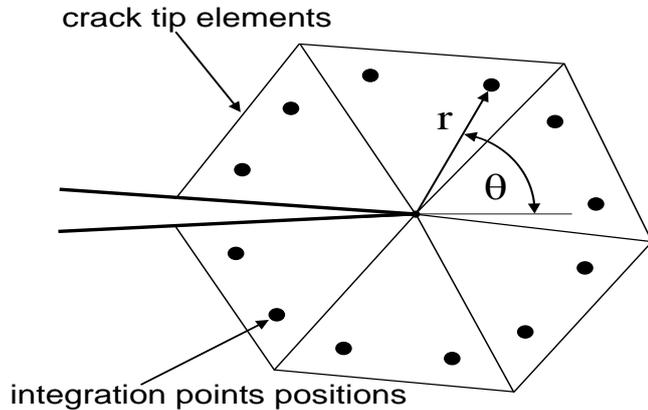
Fig. 3. Layer of integration points around crack tip
