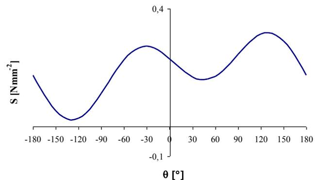
Fig. 10. Distribution of factor  $S$  round the crack tip
