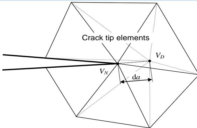
Initial and extended crack tip configuration
