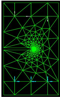
Fig. 8. Discretization of CTS specimen using finite elements
