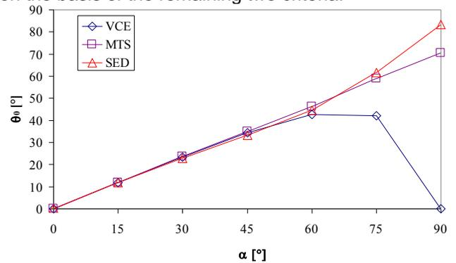
Fig. 9. Comparison of  $\theta_0$  for different criteria
