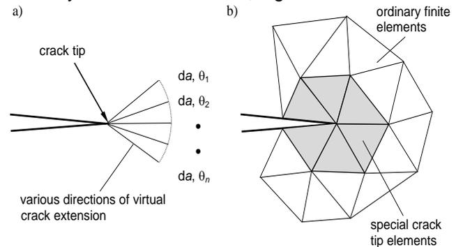
Fig. 2. Virtual crack extensions of the crack tip
