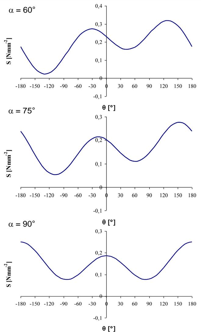
Fig. 11. Distribution of  $S$  round the crack tip, depending on the load angle  $\alpha$
