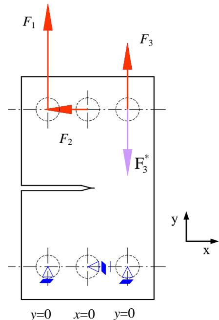
Fig. 7. Boundary conditions for CTS specimen
