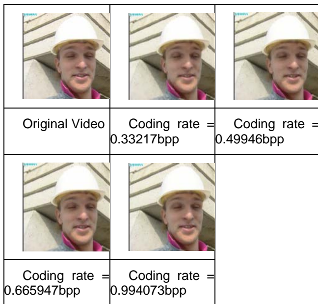
Fig. 12. Four types MPEG-2 source coding results compared with original video frame.
