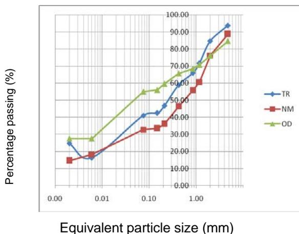
Fig. 2. Particle size distribution curves for the soil samples [16]
