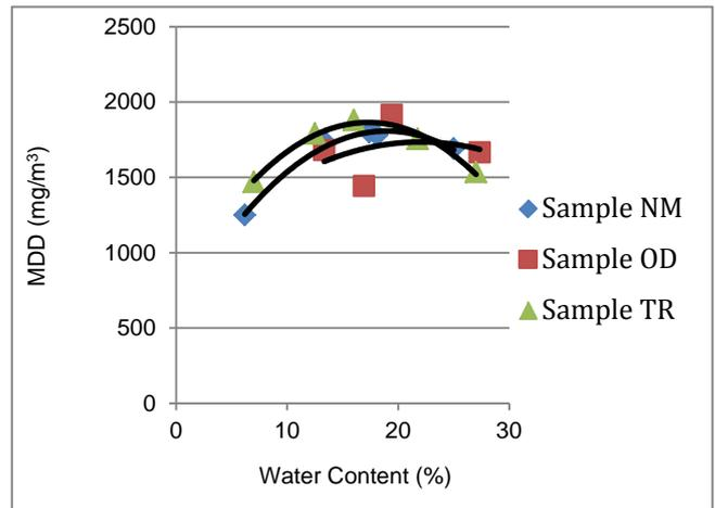
Fig.3. Compaction characteristics of the soil samples in their natural states
