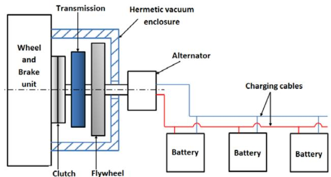
Fig. 1: Flywheel energy recovery and storage system
