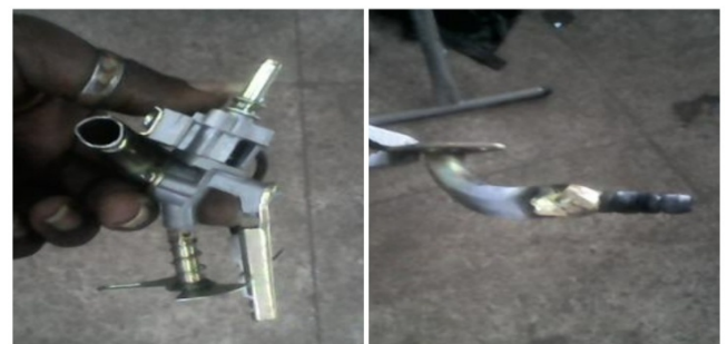
Fig 14. (L) Image of the control element, (R) welded nipple to the inlet of the control element
