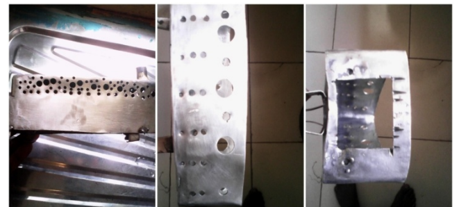
Fig 7. (L) Ventilation hole of the inner chamber. (C) Ventilation holes of the outer chamber. (R) Created passage for the control element
