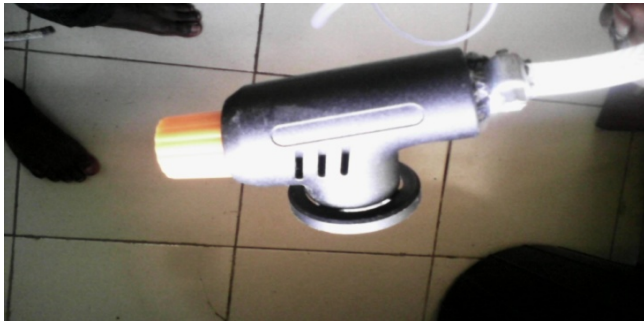
Fig 15. Image of the reconstructed flame gun with a transparent rubber hose attached to it
