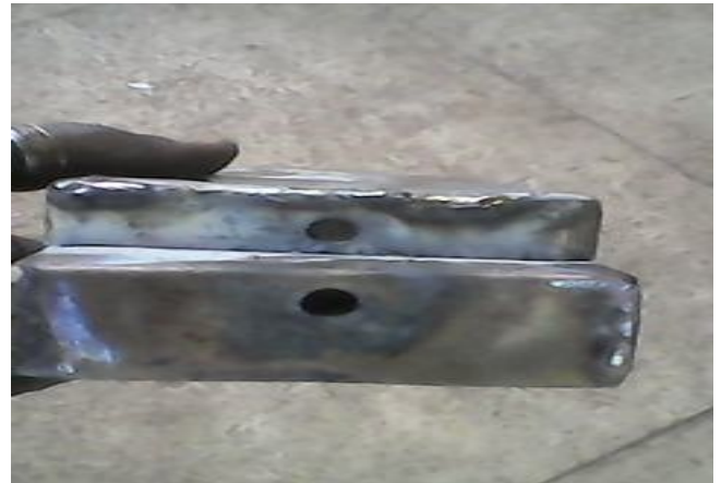
Fig 5. Image of the drilled holes at the back of the inner chamber
