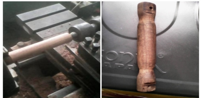
Fig 16. (L) processed cylindrical wood on a lathe machine. (R) Finished handle
