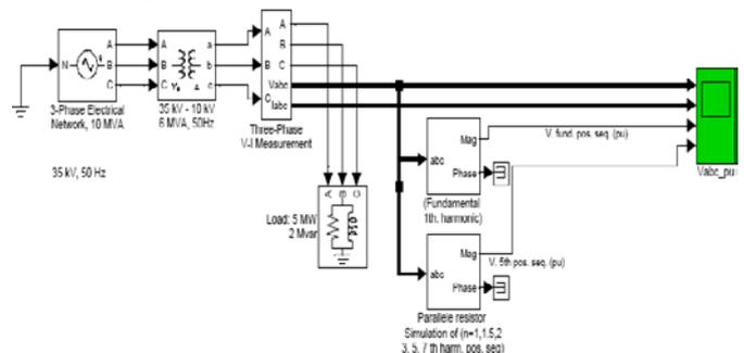
Fig. 7. Simulation signal generating n-order through the parallel sub bus power supply included a block that represents a nonlinear resistor with a time function.
