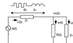
Fig. 2. Equivalent scheme that suits turning on of the device for generating signals to the network.
