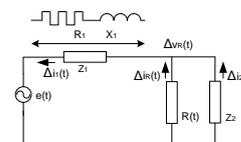
Fig. 3. Equivalent schemes and directions of electricity increment
