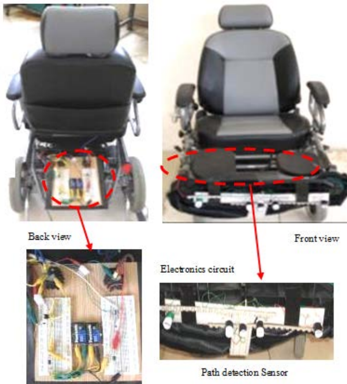
Figure 18 Physical prototype of the designed smart Mobile Robotic guidance system –Mechatronics Motawif, Mechatronics Sec. Lab., Taif University, Taif, Saudi Arabia 2012.
