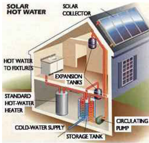
Fig. 2. Liquid-Based Solar Heating System, [5]
