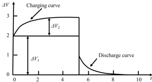
Fig. 1. Schematic diagram of the induced polarization phenomenon in the time domain
