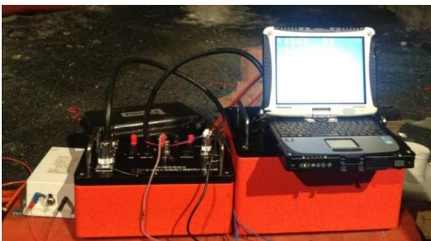
Fig. 2. The advanced prediction instrument
