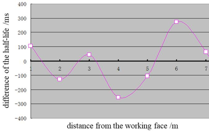
Fig. 4. Detection result of the difference in the half-life of the excitation polarization of a certain detection
