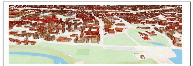
Fig. 4. Building volumes derived from LiDAR point cloud.
