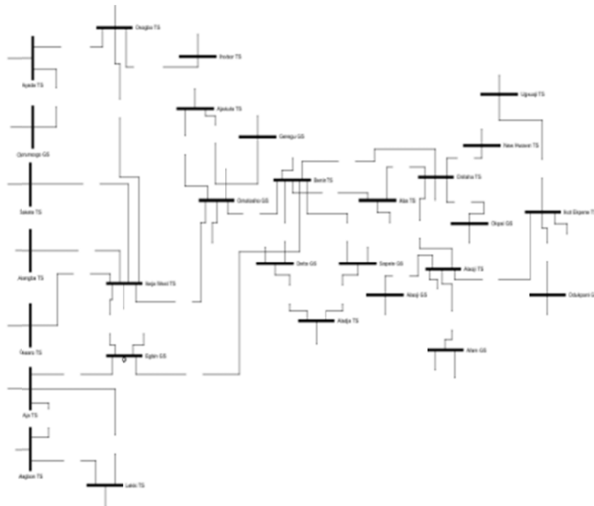
Figure 3.5: Modelled 330 kV Network Without FACTS Integration
