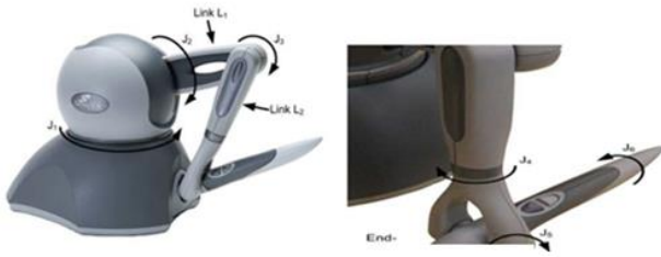
Figure 7: PHANTOM Omni Showing Actuated and Non-Actuated Joints [34]
