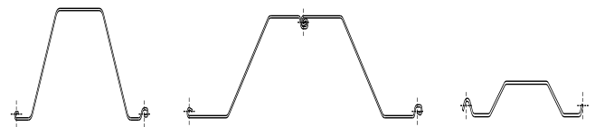
Fig. 1 Sheet pile typical sections
