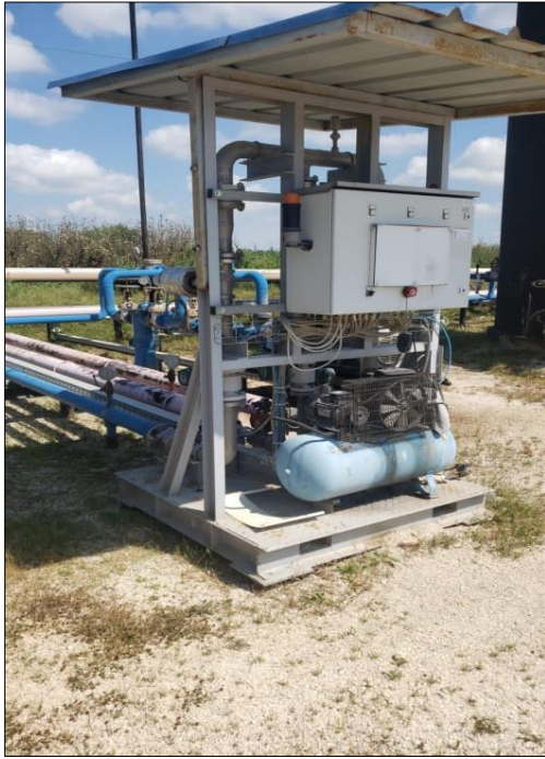
Figure 8. The PDU unit remotely monitors fluid filtration to improve injection quality (Photo: author 2022)
