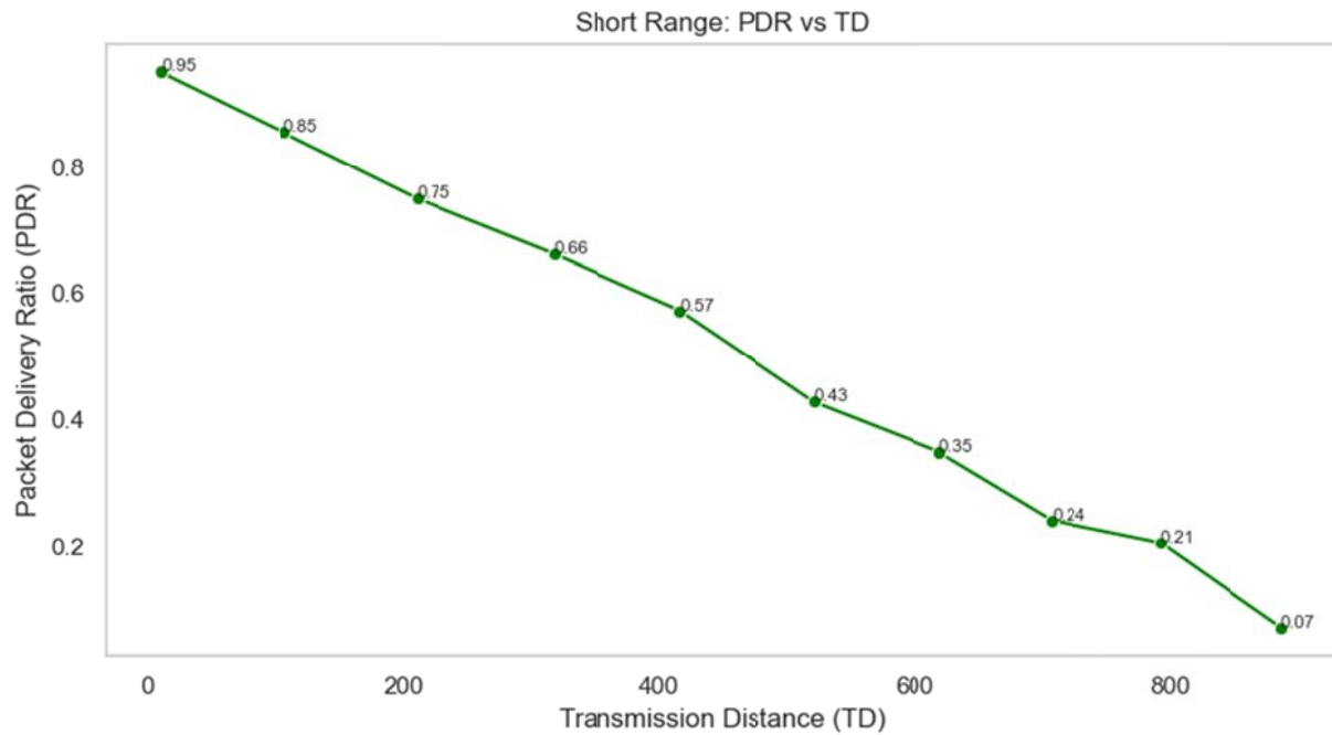
Figure 2: The PDR at the optimal parameter configuration
