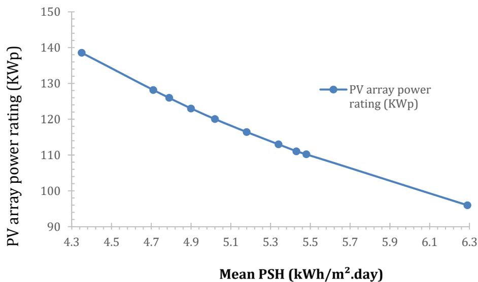
Figure 4 The graph of PV array power rating (KWp) versus mean PSH (kWh/m<sup>2</sup>.day)
