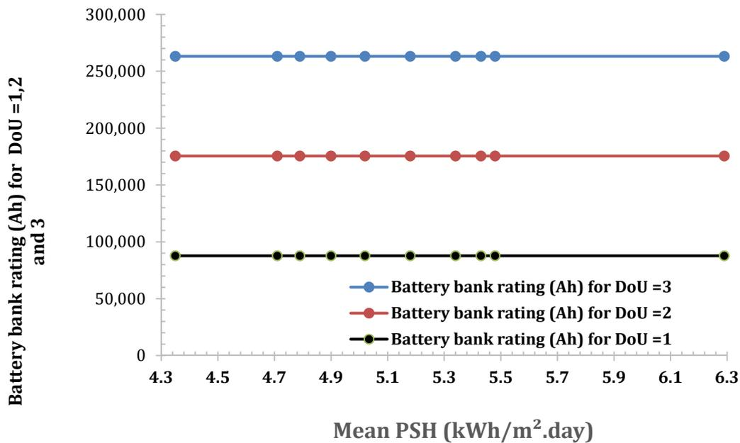
Figure 5 The graph of battery bank rating (Ah) for DoU =1,2 and 3 versus mean PSH (kWh/m<sup>2</sup>.day)
