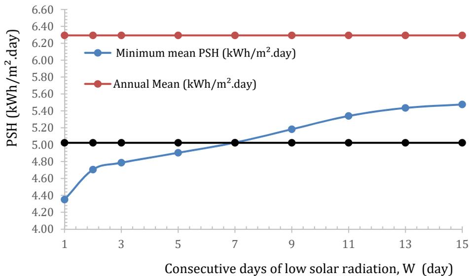
Figure 2 The minimum mean PSH (kWh/m<sup>2</sup>.day) for different consecutive days of low solar radiation, W (day)
