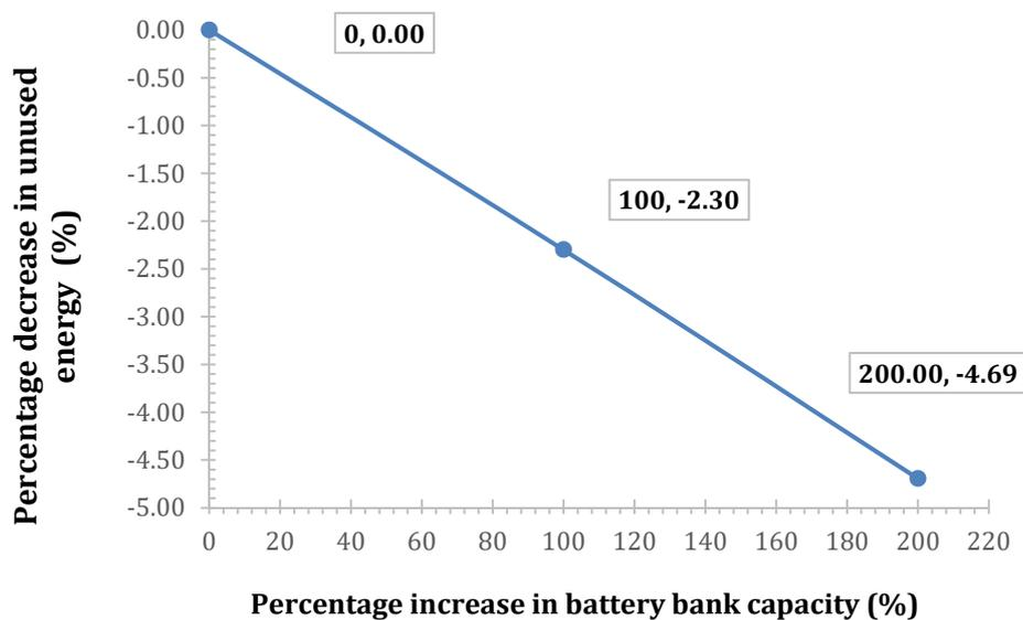
Figure 7 Percentage decrease in unused energy (%) versus Percentage increase in battery bank capacity (%)
