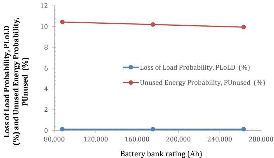
Figure 6 Loss of Load Probability, PLoLD (%) and Unused Energy Probability, PUnused (%) versus Battery bank rating (Ah)
