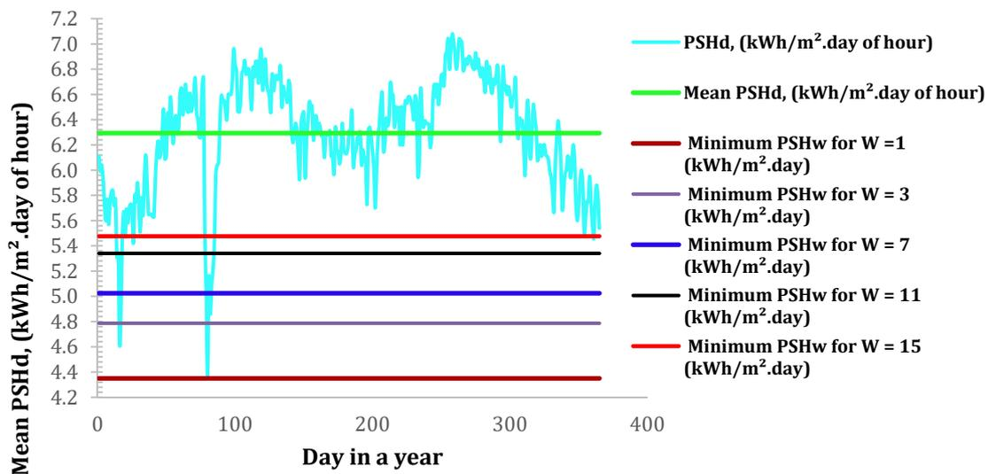
Figure 3 The solar radiation data of Akwa Ibom State with annual mean of the daily peak sun hour and minimum mean PSH for different consecutive days of low solar radiation, W
