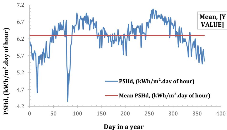
Figure 1 The solar radiation data of Akwa Ibom State with annual mean of the daily peak sun hour of 6.2933 kWh/m<sup>2</sup>.day or hours/day
