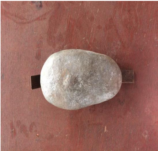
Fig 10: Zinc Sacrificial Anode
