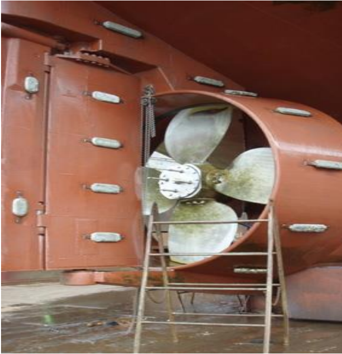
Fig 13: Sacrificial Anodes attached to a ship
