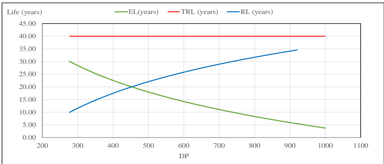
Fig. 2. Transformer Lifetime Operation (TRL), Elapsed Transformer Life (EL), and Remaining Life (RL), as a Function of the Degree of Polymerization (DP)
