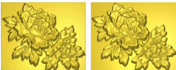
3D model of the original grayscale image Smooth original grayscale image 3D model
