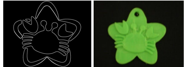
(a) The contour curve loops (b) 3D printer finished product
