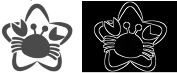
(a) Image after Gaussian filtering (b) Image after Sobel filter Figure 4 The edge of the image processed by the Sobel filter.
