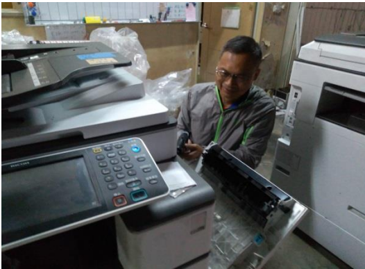
Fig. 4. Detecting the asymmetric motor of the laser exposure group
