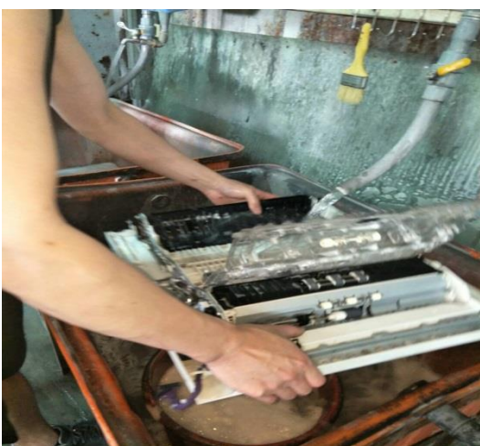
Fig. 6 Repaired the laser exposure group
