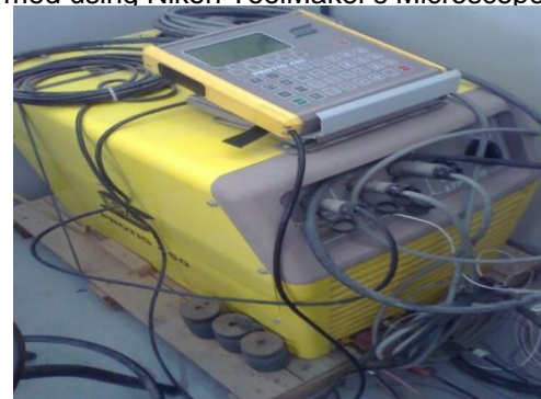
FIGURE I. TIG MACHINE POWER SUPPLY
