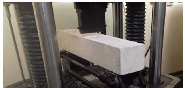
Fig. 4: Experimental test set-up for beam specimens
