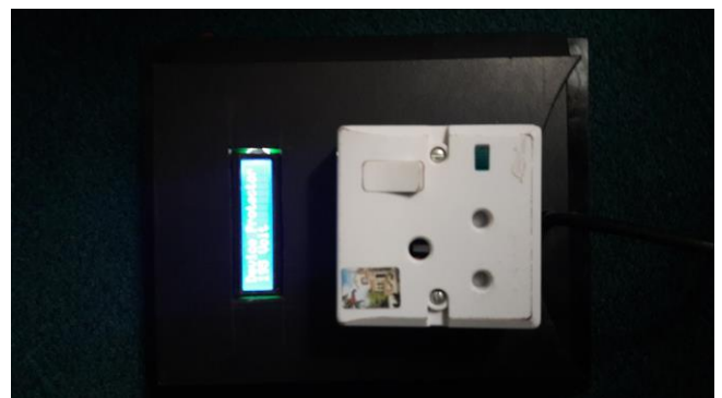
Figure 7: Photograph of the protective device when connected to the mains
