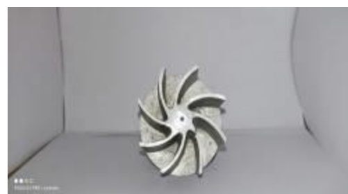
Fig. 8. semi-open impeller with 6 blades.
