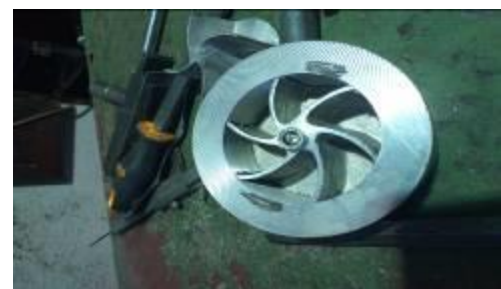
Fig. 7. semi-open impeller with 6 blades.
