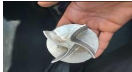
Fig. 6. semi-open impeller with 4 blades.
