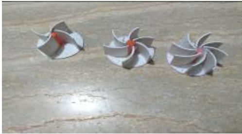
Fig. 9. semi-open impellers with 4, 6 and 8 blades.
