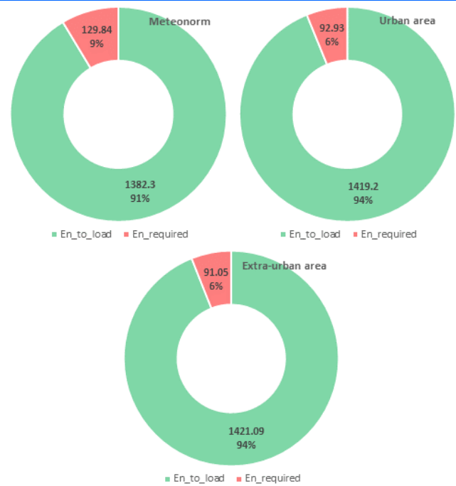
Fig. 5. Annual values of energy to load obtained from the simulations using Meteonorm weather databases and measured weather data for the urban and extra-urban area of Braşov
