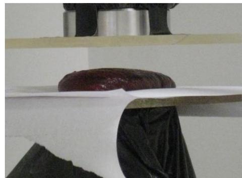
Fig. 1. Human spleen placed between the compression plates of an MTS
