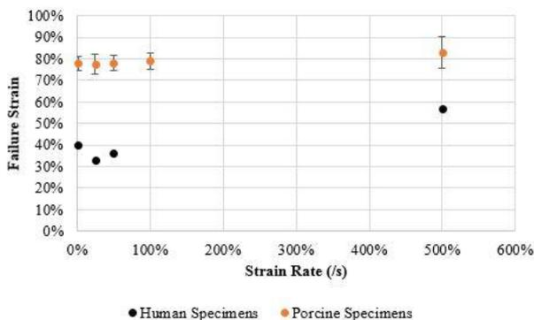
Fig. 7. Failure strain of porcine spleen at various rates under unconfined compression
