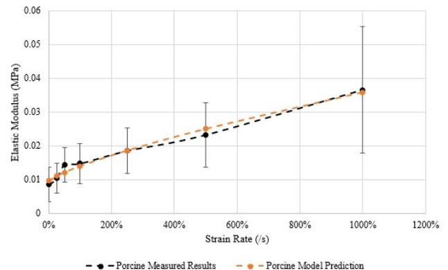
Fig. 5. Measured and modeled elastic modulus of the porcine specimens at different strain rates
