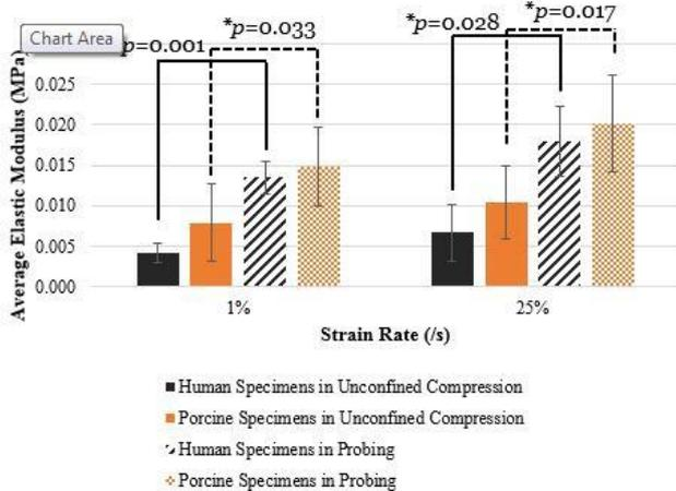
Fig. 4 Porcine human and porcine measured and modeled elastic modulus of the porcine specimens at different strain rates.
