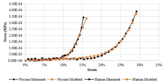
Fig. 3. Representative measured and modeled stress-strain curves of the human and porcine spleen in unconfined compression at a rate of 25%/s
