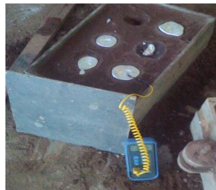
Figure 3: Measuring the cooling rate of molten Al alloy
