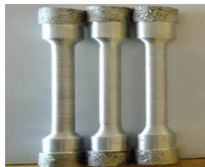
Figure 4: Machined tensile test specimen
