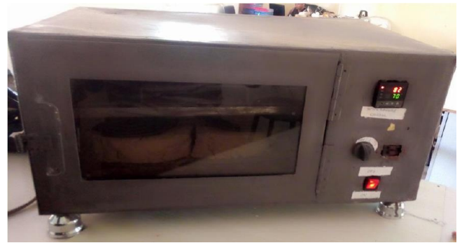
Fig. 2: The developed electric cocoa-bean dryer. The solar power unit is at the back of the dryer.
