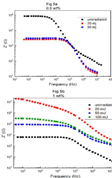
Figure 5 (a and b): The variation of the SWCNTs/PMMA samples imaginary part of impedance with frequency for different laser treatment doses.
