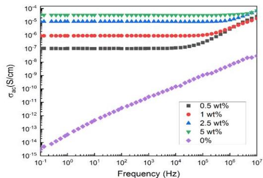
Figure (1): Dependence of the ac. Conductivity of pristine PMMA and its composites filled with non-irradiated SWCNT.
