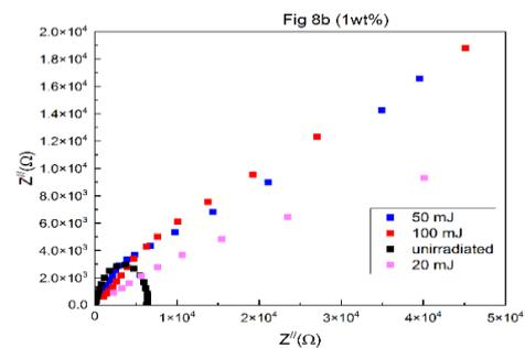
Figure 8: Cole-Cole Plots for samples loaded with 0.5wt% and 1.0 wt% of CNTs and treated with different doses of laser at room temperature.
