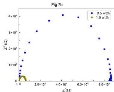
Figure 7: The Cole-Cole Plots of all untreated SWCNTs/PMMA composites at room temperature.
