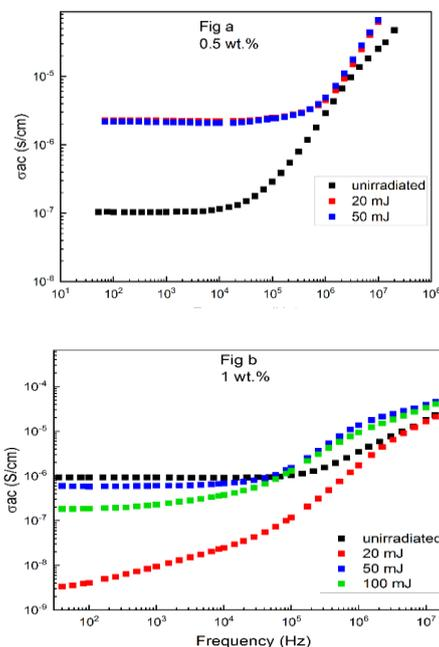
Figure 3: Frequency dependence of ac conductivity,  $\sigma_{ac}$  for laser treated SWCNTs/PMMA samples at room temperature.
