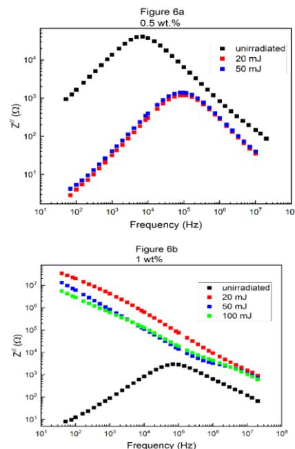
Figure 6 (a and b) : The variation of the SWCNTs/PMMA samples imaginary part of impedance with frequency for different laser treatment doses.
