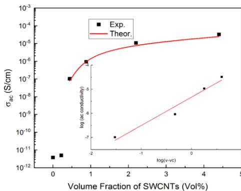
Fig. 2: Dependence of ac electrical conductivity of PMMA loaded with different volume fractions of SWCNTs at room temperature and 100Hz.
