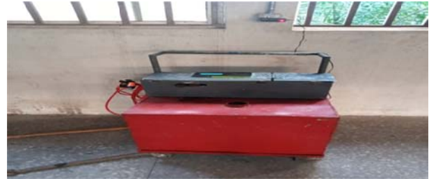
Figure 10: The Fabricated Mobile Water Sprayer
